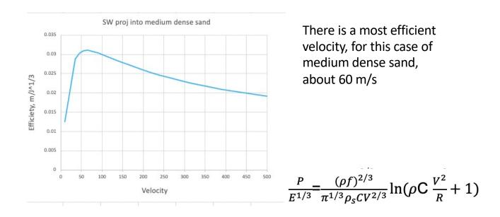
With constant velocity constraint, penetration scales as fineness ratio and density  $^{2/3}$ .
