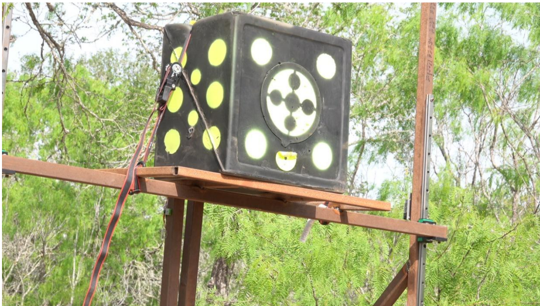
Target mounted on a free-fall drop system used to simulate reaction timing.
