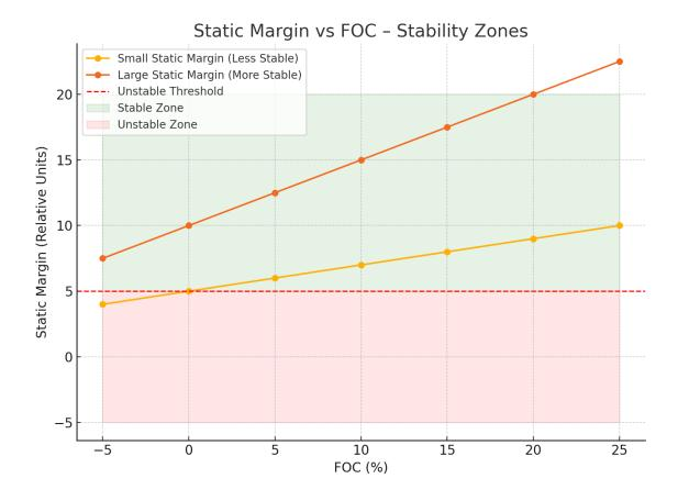
The chart shows how static margin increases with F.O.C. when the center of pressure (CP) is fixed. The 'Large Static Margin' line represents arrows with CP positioned far behind the CG (usually due to large rear vanes), resulting in more stability across all F.O.C. levels. The 'Small Static Margin' line represents arrows where CP is closer to CG, creating a narrow margin and less stability unless F.O.C. is significantly increased.
